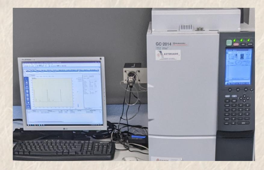
Figure 2. Gas chromatography utilised to estimate the methane production of the digesters
